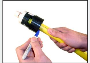
**6** If using ID chamfer tool with gauge, check for proper chamfer by inserting pipe on gauge up to the o ring. With proper chamfer, o ring will begin to enter pipe.
