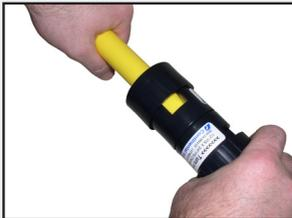
**5** Mark the stab depth by inserting pipe into ID chamfer tool and marking the pipe at the entrance as shown.
